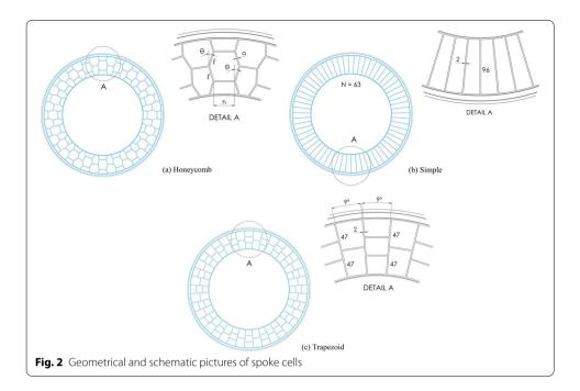
where  $E_r^*$ ,  $E_{\cap}^*$ , and  $G_{r\cap}^*$  are the effective modulus values in the radial, circumferential, and shear directions. As shown in Fig. 2a, the  $\theta$ , l and h represent the values of the spokes cell angle, cell inclined length, and vertical length of the cell. The 'a' represents the cell wall thickness as shown in Fig. 2 and  $E_s$  represents the value of the base material's young modulus.
