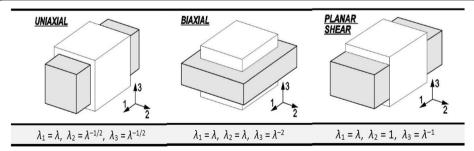
Fig. 4 Uniaxial, biaxial, and planar shear deformation modes and relationships between the elongations
