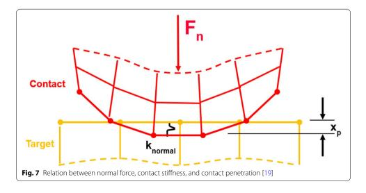
contact force (pressure) calculations. The  $k_{\rm normal}$  stiffness value is a very important variable that affects both the convergence phenomenon as well as the accuracy of the analysis. When we use large values of stiffness,  $k_{\rm normal}$  the accuracy of the analysis is increased but the analysis may have some difficulties in converging the solution.
