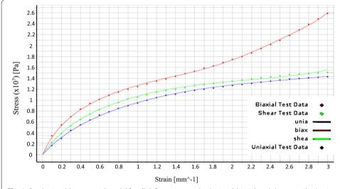
**Fig. 6** Synthetic rubber material model for all deformation modes (uniaxial, biaxial, and shear test data) using MR 9 parameter model to evaluate the  $C_{ij}$  constants
