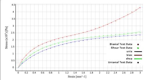
**Fig. 5** Polyurethane material model for all deformation modes (uniaxial, biaxial, and shear test data) using MR 9 parameter model to evaluate the  $C_{ij}$  constants
