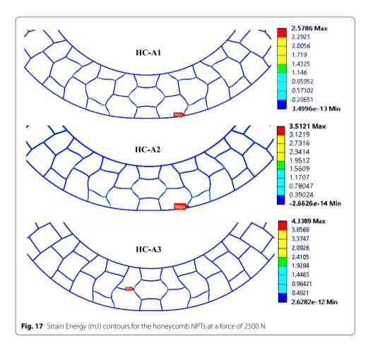
modulus of elasticity  $E_r/E_s = 0.02$ , the value of HC-A3 is high, that is why it has a high value of strain energy (mJ).
