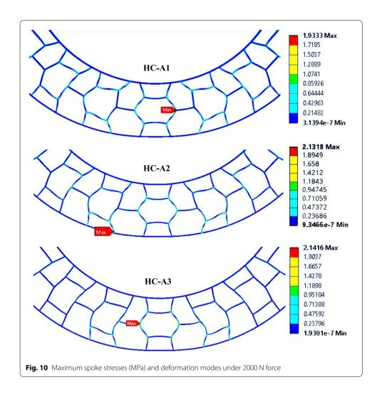
The lower local stresses and lower strain energy values in the spokes of the simple and HC-A1 structures are much better for the designing of the fatigue-resistant NPTs spokes. The trapezoid spoke structure can absorb the maximum amount of energy when deformed under vertical loading because it has the maximum value of strain energy, so it can be used in many of the energy absorbing structure applications.
