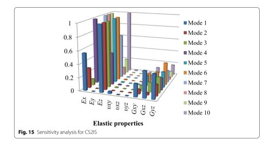
with a single stiffener in the transverse direction with a 5% increment in the individual elastic parameters.
