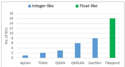
**Fig. 17** No. of quantized bits that resulted in the best performance for the GAN undertest. Each technique is tested on different GAN. The works QGAN [46], QMGAN [49], GanSlim [37], Flexpoint [52], and TGAN [51] are fully quantized. While ApGan [50] has mixed quantized and non-quantized layers. Also, FlexPoint, ApGAN and TGAN quantization is used during training
