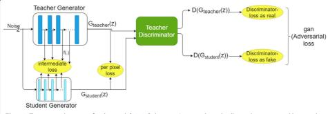
Fig. 10 Training architecture for the work [28, 30] showing Intermediate distillation loss, per-pixel loss, and GAN loss
