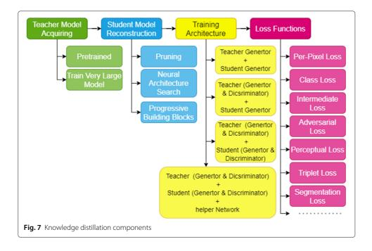
The last component is the loss function. The loss function determines how good and how fast the student will learn from the teacher. A lot of loss function has been introduced that will be explained below.
