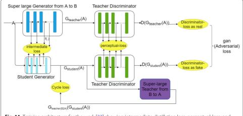
Fig. 11 Training architecture for the work [33] showing intermediate distillation loss, perceptual-loss, and gan-loss
