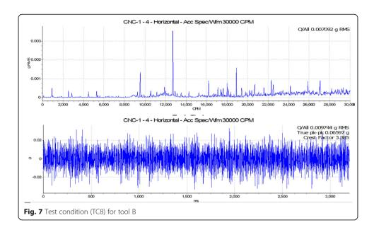
The depth of cut, feed, and speed are varied for both the tools and measuring velocity at horizontal and axial alongside with horizontal and axial accelerations, since for measuring, the vibrations generated accurately the horizontal vibrations, which are considered for better understanding. The vibrations recorded are in Table 3 and Table 4 for tool A and tool B, respectively.
