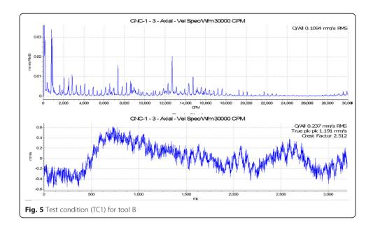
restrictions are well thought out, and VB 0.3 mm is treated as a cutoff value for drilling activity. To determine the state of the tool-based vibration frequency, the displacement parameter value  $\leq 60\,\mu m$  and RMS velocity of the spinning object  $\leq 4.5\,mm/s$  along with acceleration are used in compliance with ISO 10816-3 requirements for vibration intensity.
