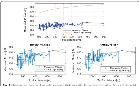
**Fig. 7** Measured propagation loss estimation and their error distribution statistics using classical Egli model and adapted *Egli model* for Cell\_4
