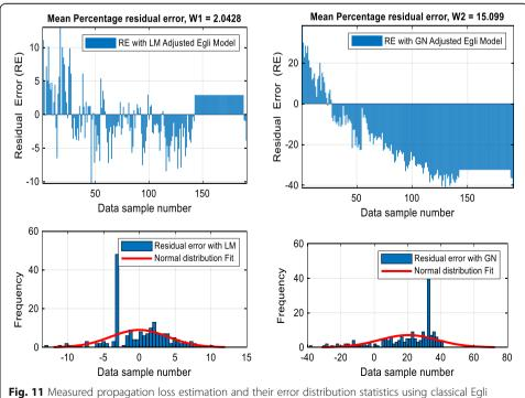
**Fig. 11** Measured propagation loss estimation and their error distribution statistics using classical Egli model and adapted *Egli model* for Cell\_4
