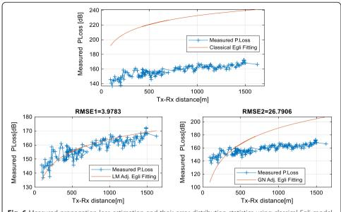
**Fig. 6** Measured propagation loss estimation and their error distribution statistics using classical Egli model and adapted *Egli model* for Cell\_3
