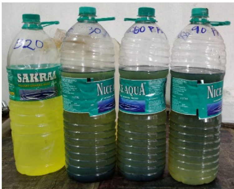
Fig. 9 Blends of Moringa methyl ester (MME20, MME20 + 30 ppm, MME20 + 60 ppm, MME20 + 90 ppm)
