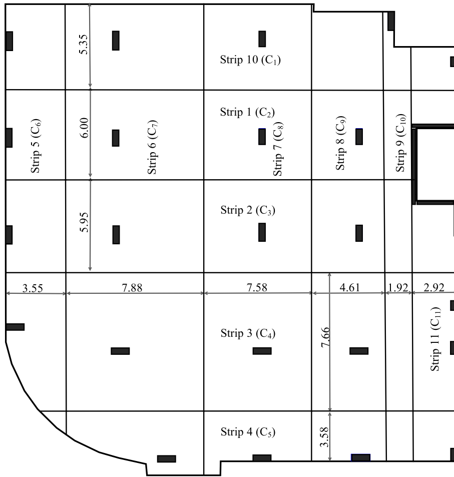
Fig. 7 Design strips and cables numbering in Example 1
