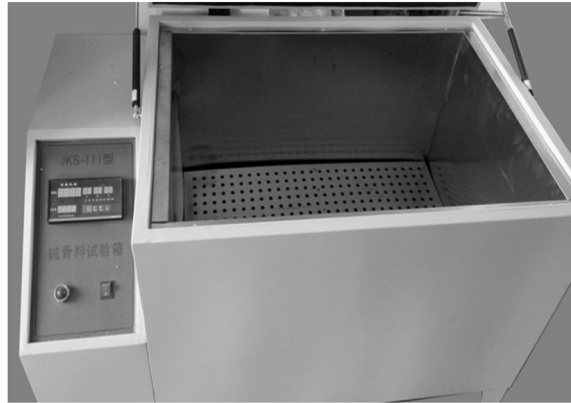
Fig. 2 Structure diagram of AST asphalt mixture standard tester
