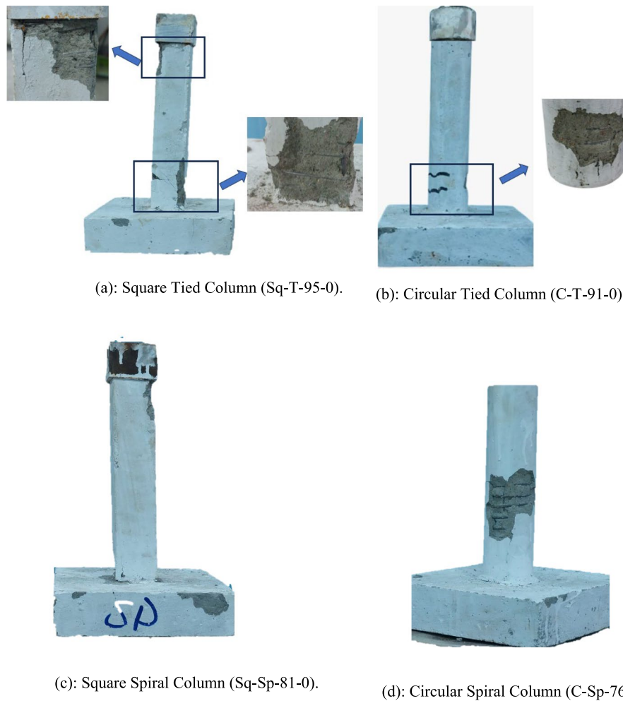
Fig. 10 The failure mode of Group 2 specimens. a Square tied column (Sq-T-95-0). b Circular tied column (C-T-91-0). c Square spiral column (Sq-Sp-81-0). d Circular spiral column (C-Sp-76-0)
