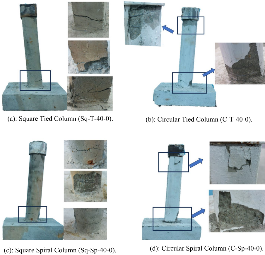
Fig. 13 The failure mode of Group 3 specimens. a Square tied column (Sq-T-40-0). b Circular tied column (C-T-40-0). c Square spiral column (Sq-Sp-40-0). d Circular spiral column (C-Sp-40-0)
