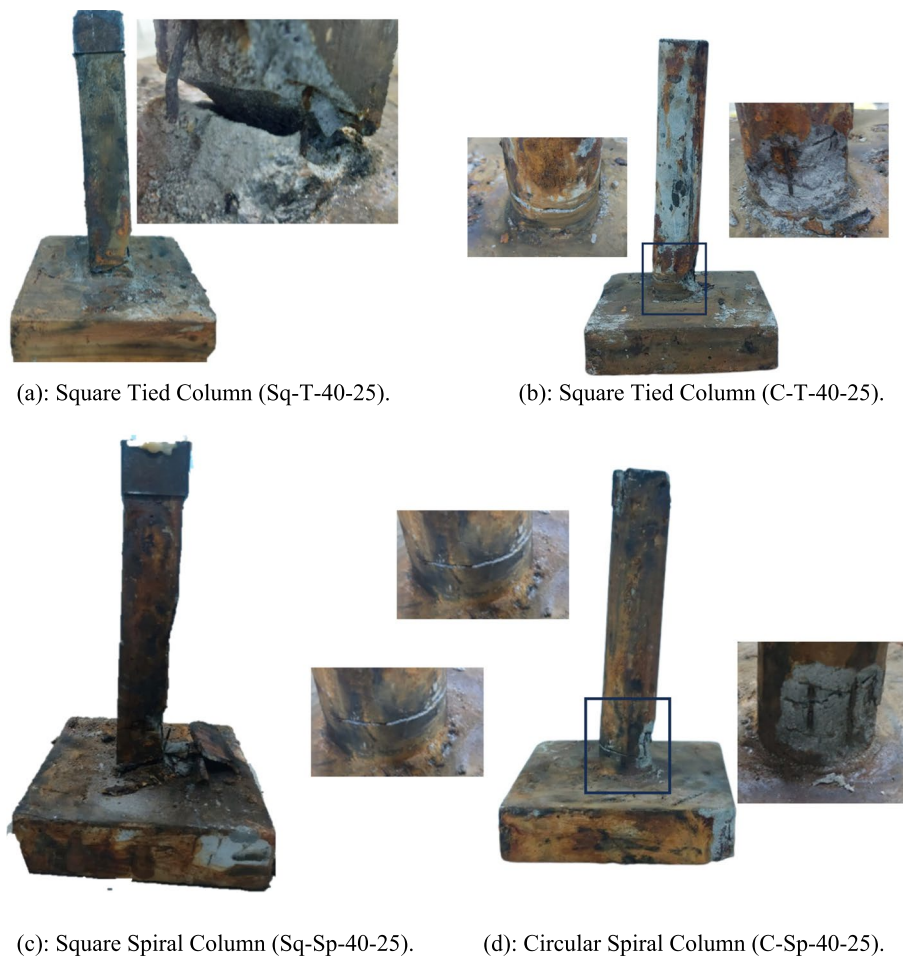
Fig. 19 The failure mode of Group 5 specimens. a The horizontal load-lateral drift curve for specimen (Sq-T-40-25). b The horizontal load-lateral drift curve for specimen (C-T-40-25). c The horizontal load-lateral drift curve for specimen (Sq-Sp-40-25). d The horizontal load-lateral drift curve for specimen (C-Sp-40-25)
