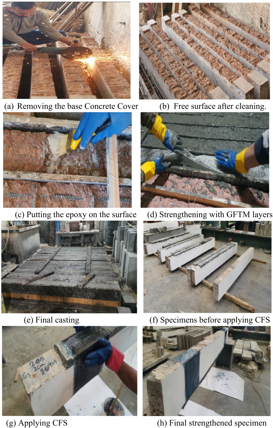
Fig. 8 Strengthening processes in laboratory
