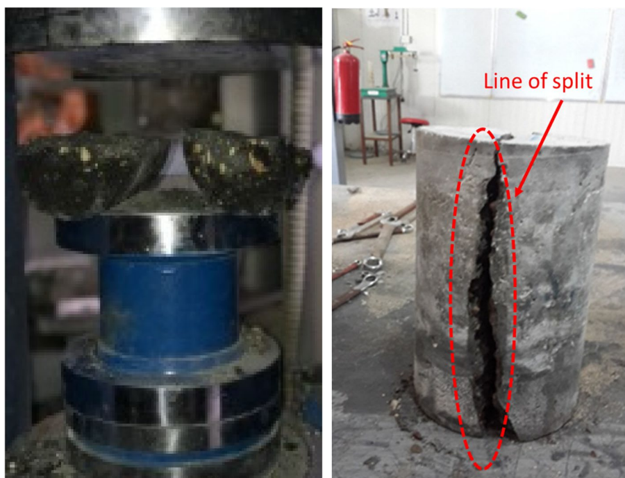
Fig. 13 Shows the failure mode of concrete prism after exposed to test in split
