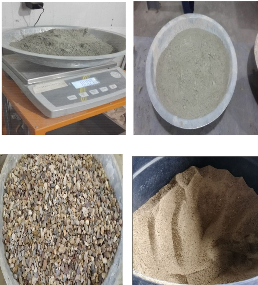
Fig. 3 Materials used in the experimental work for concrete production
