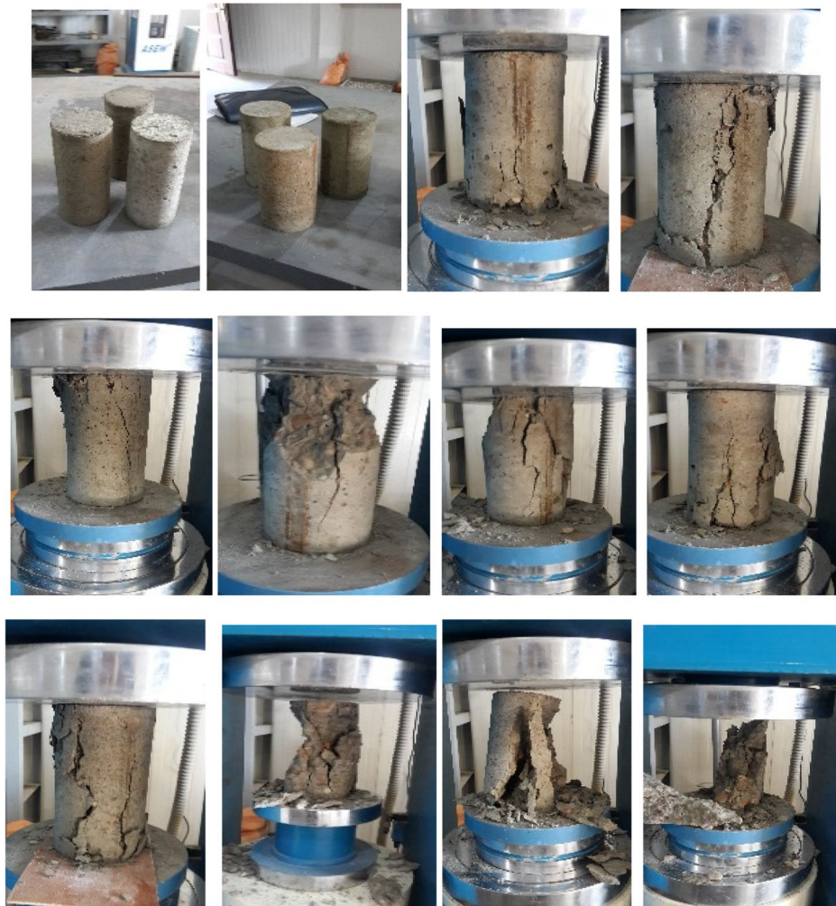
Fig. 10 Shows the failure mode steps of concrete cylinders after being exposed to test in compression
