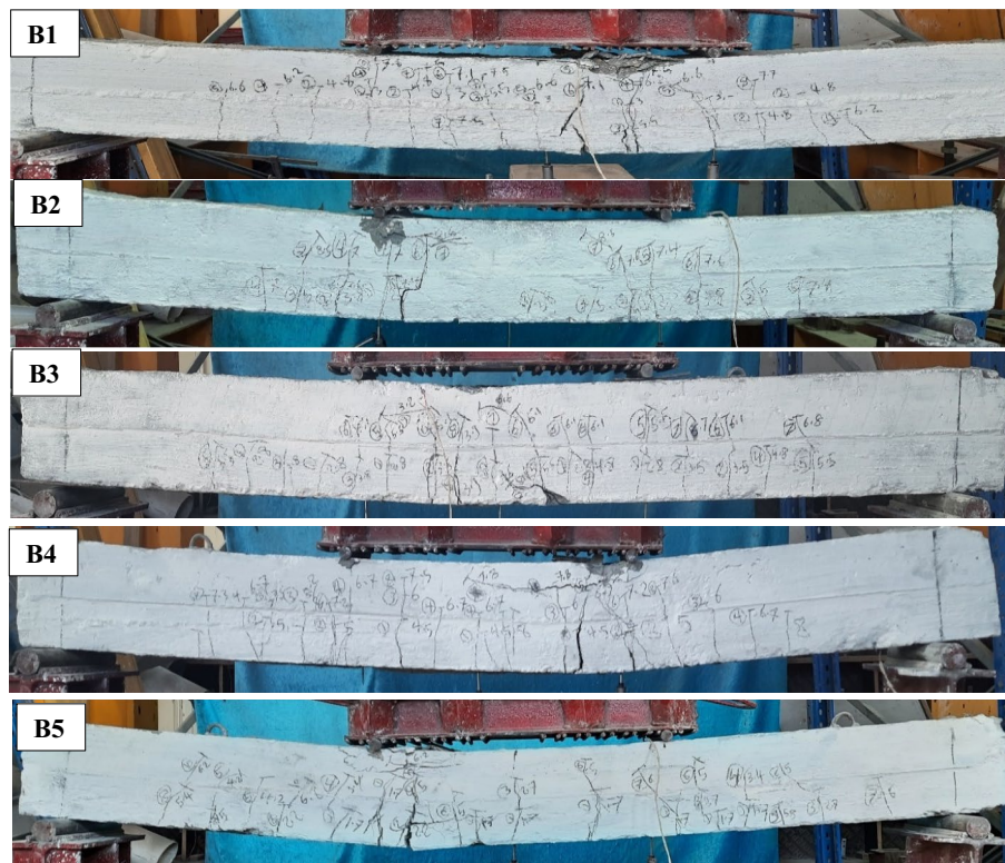
Fig. 13 Crack pattern for all tested beams
