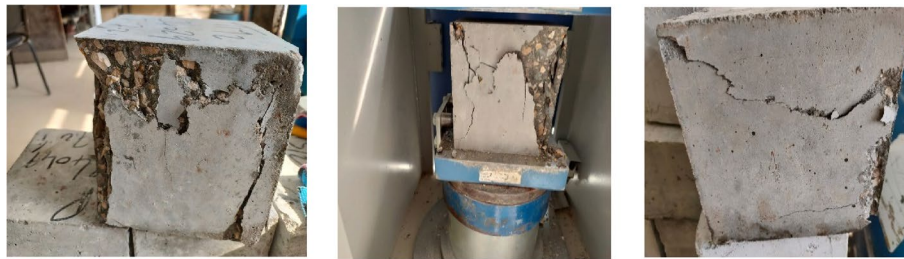
Fig. 5 Mode of failure of cubes
