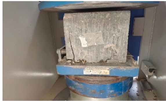
Fig. 4 Test setup for compression test
