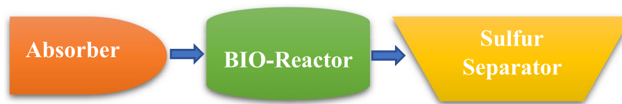
Fig. 7 Block diagram of the main sections of THIOPAQ
