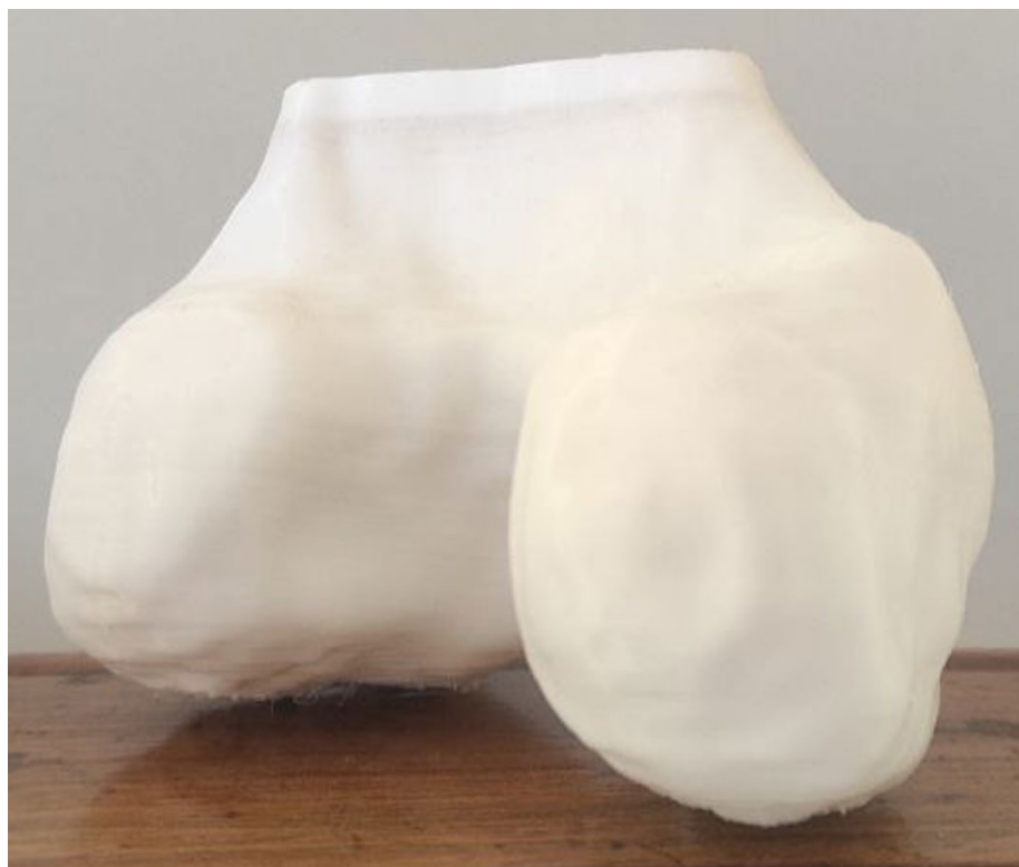
Fig. 9 3D printed model of the distal femur bone using optimum parameter
