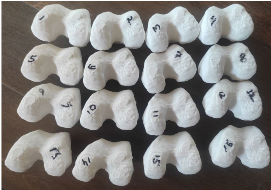
Fig. 5 3D printed distal femur bone as per the experimental layout of L_{16} orthogonal array
