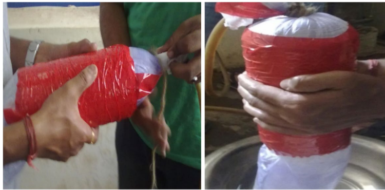
Fig. 4 a, b PC preparation for permeability test
