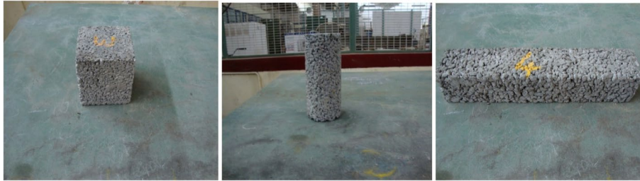
Fig. 1 a–c Cube, cylindrical, and prism specimen for compressive, splitting tensile, and flexural tensile tests
