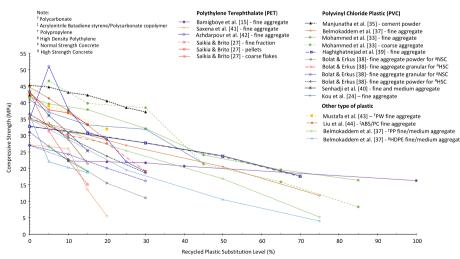
Fig. 9 Compressive strength of concrete with various type of plastic at 28 days
