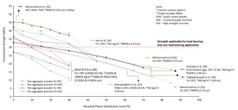
Fig. 8 Compressive strength of concrete with PVC plastic waste at 28 days
