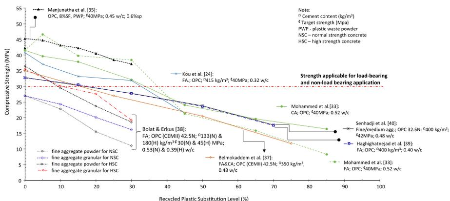
Fig. 8 Compressive strength of concrete with PVC plastic waste at 28 days
