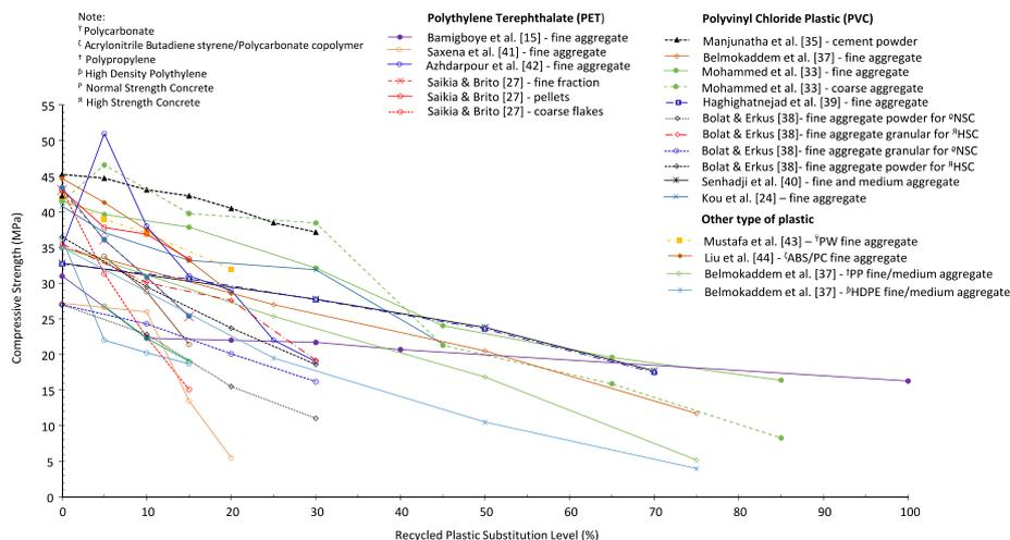
**Fig. 9** Compressive strength of concrete with various type of plastic at 28 days
