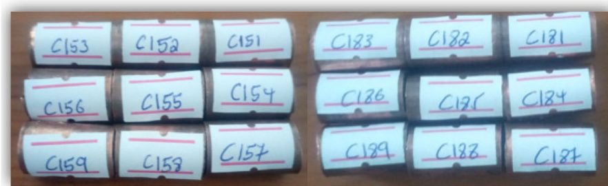
Fig. 3 Experimental sample after turning CuZr and CuCrZr
