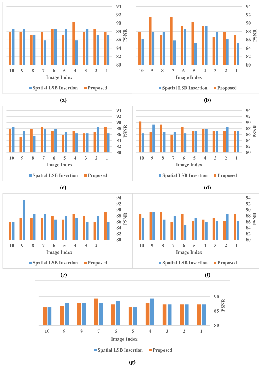
Fig. 4 PSNRs for the BOSS database/proposed LSB technique with different message sizes with 4 \times 4 block size. a Message size = 4 KB, b message size = 6 KB, c message size = 8 KB, d message size = 10 KB, e message size = 12 KB, f message size = 14 KB, and g message size = 16 KB
