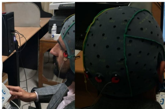
Fig. 1 Electrode placement positions for SSVEP (right) and HEOG (left) recording
