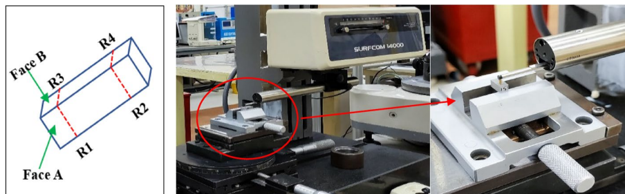
Fig. 18 a Surface roughness measurement technique. b Surfcom roughness tester. c Enlarged view of working zone of tester
