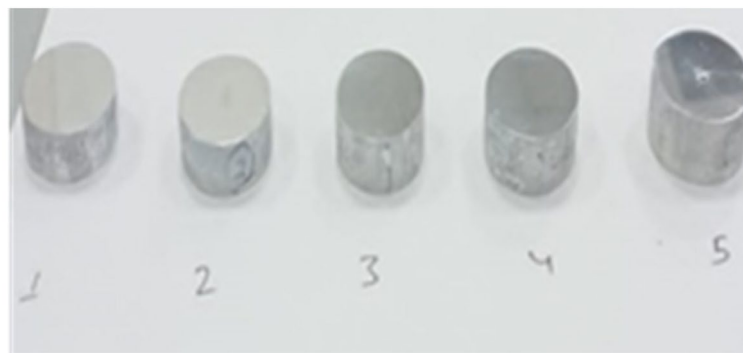
Fig. 5 Sample for OM, SEM, and hardness test
