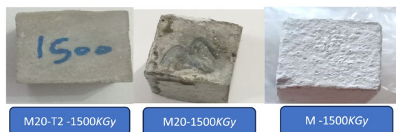
b: visual appearance of various samples after irradiating by 1500KGy
