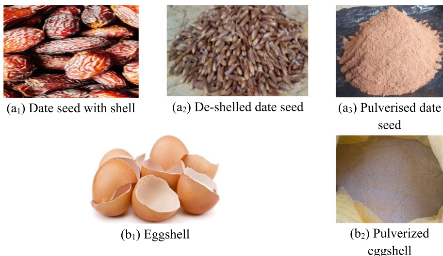
Fig. 1 Pulverization of date seed and eggshell. a 1 Date seed with shell. a 2 De-shelled date seed. a 3 Pulverized date seed. b 1 Eggshell. b 2 Pulverized eggshell
