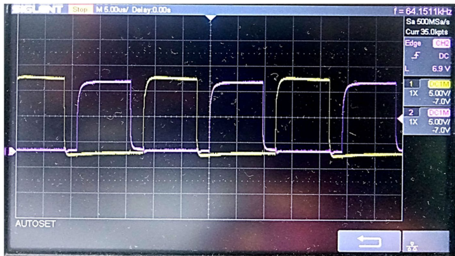
Fig. 17 IGBT Gate pulses obtained from driver circuit based on high-speed opto-coupler
