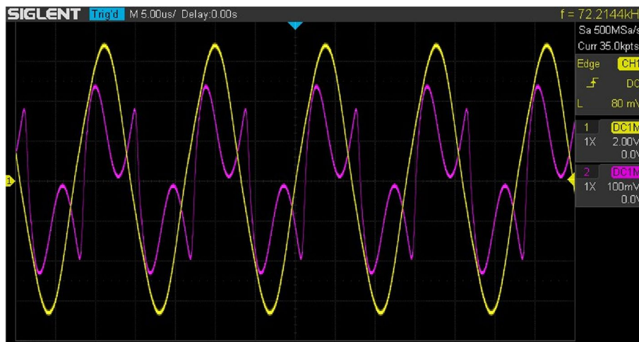
Fig. 8 Resonant current (yellow) and inverter current (pink) of parallel resonant induction heater
