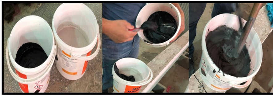
Fig. 1 The mixing of component A and B of the adhesive material
