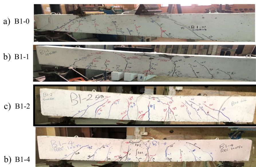
Fig. 8 Crack pattern for beams without CFRP laminates
