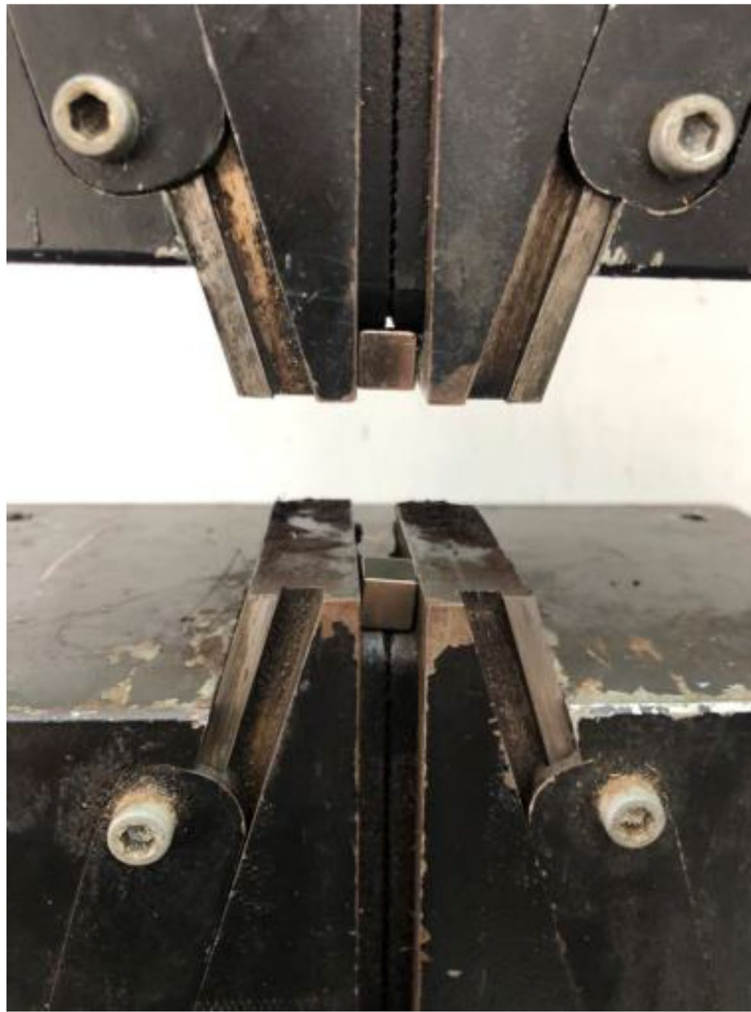
Fig. 4 Experimental measurement of the magnetic force using the UTM
