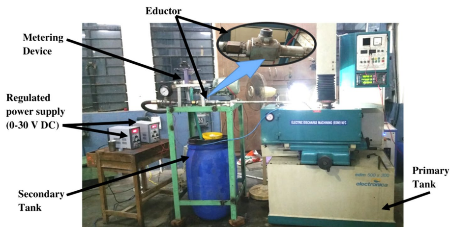
Fig. 1 Arrangement of the experimental setup for the newer mixing method in PMEDM system
