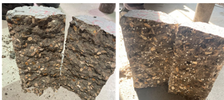
Fig. 12 Tensile strength failure for samples a PET, b HDPE
