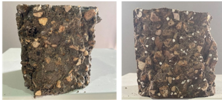
Fig. 10 Compression failure for concrete samples with a PET and b HDPE
