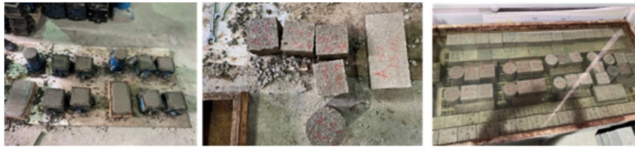
Fig. 4 Samples demoulding and curing
