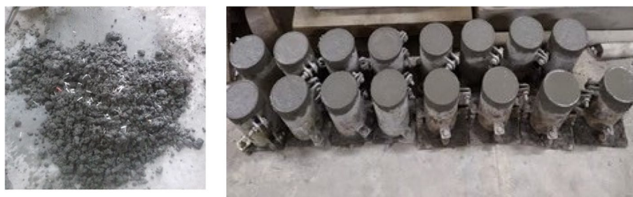
Fig. 3 Preparation of concrete specimens
