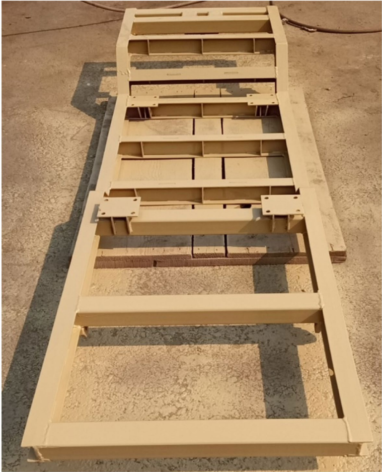
Fig. 13 The structure of the equivalent chassis after assembling, welding, and painting processes
