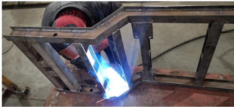
Fig. 12 The welding process of the I-shape cross-members with the chassis
