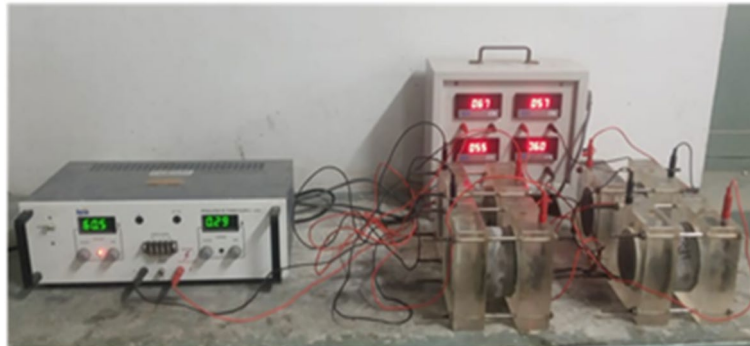
Fig. 2 Rapid chloride penetration test arrangements
