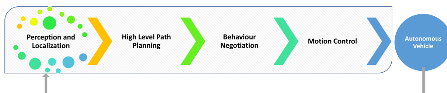
Fig. 1 Broad architecture of a perception, planning, and control workflow in autonomous vehicles
