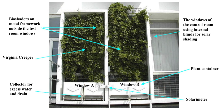
Fig. 5 Bioshader wall in the summer [18]. The units of windows are not covered with plants, and others are covered with plants and the utilized equipment to carry out the Bioshader experiment
