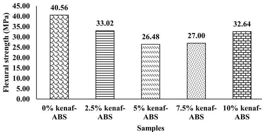
**Fig. 7** Flexural strength for kenaf-ABS composites
