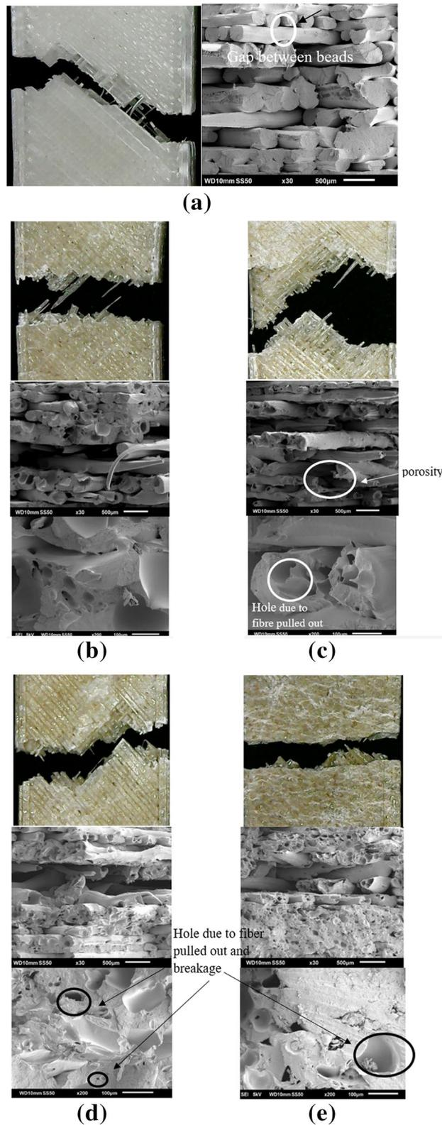
**Fig. 5** Visual picture and SEM for tensile test (a) 0% kenaf-ABS (b) 2.5% kenaf-ABS (c) 5% kenaf-ABS. Visual picture and SEM for tensile test (d) 7.5% kenaf-ABS (e) 10% kenaf-ABS
