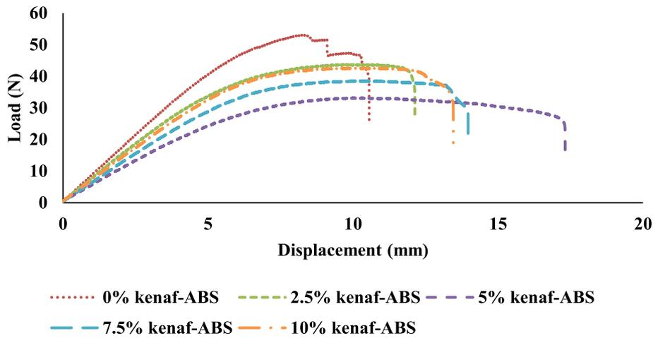
**Fig. 6** Load versus displacement for flexural testing
