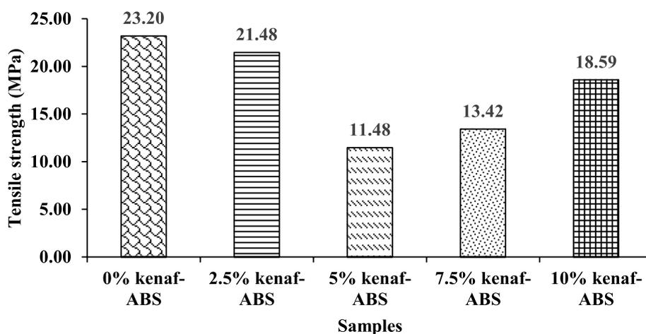
**Fig. 3** Tensile strength for kenaf-ABS composites
