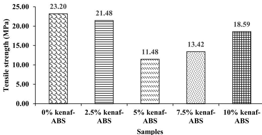
**Fig. 3** Tensile strength for kenaf-ABS composites
