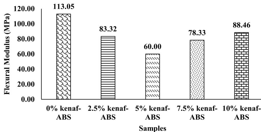
**Fig. 8** Flexural modulus for kenaf-ABS composites
