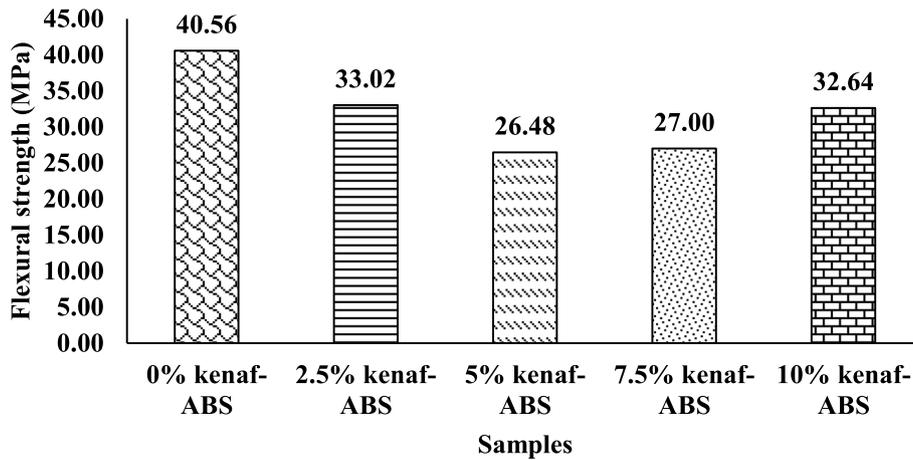
**Fig. 7** Flexural strength for kenaf-ABS composites
