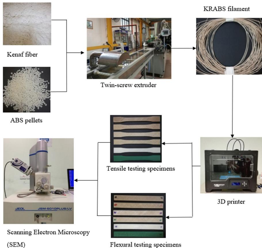
**Fig. 1** Fabrication and testing process
