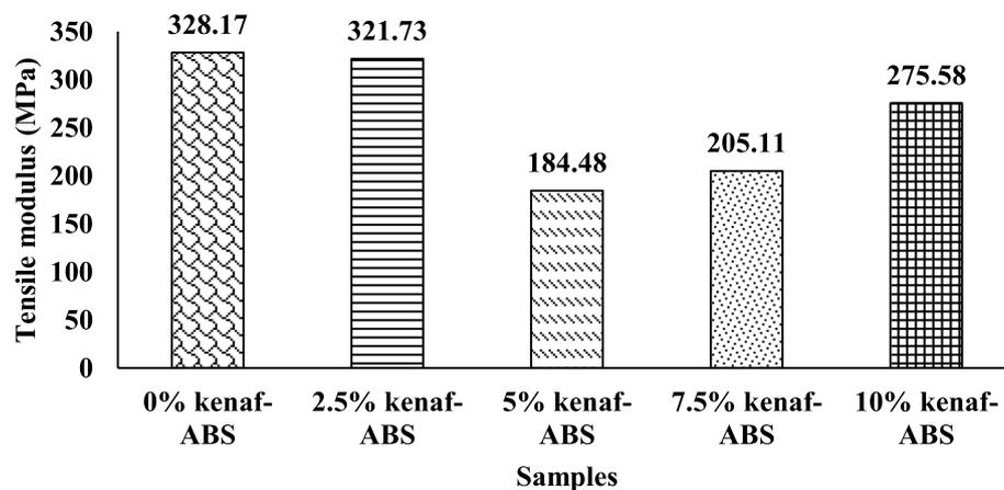
**Fig. 4** Tensile modulus for kenaf-ABS composites
