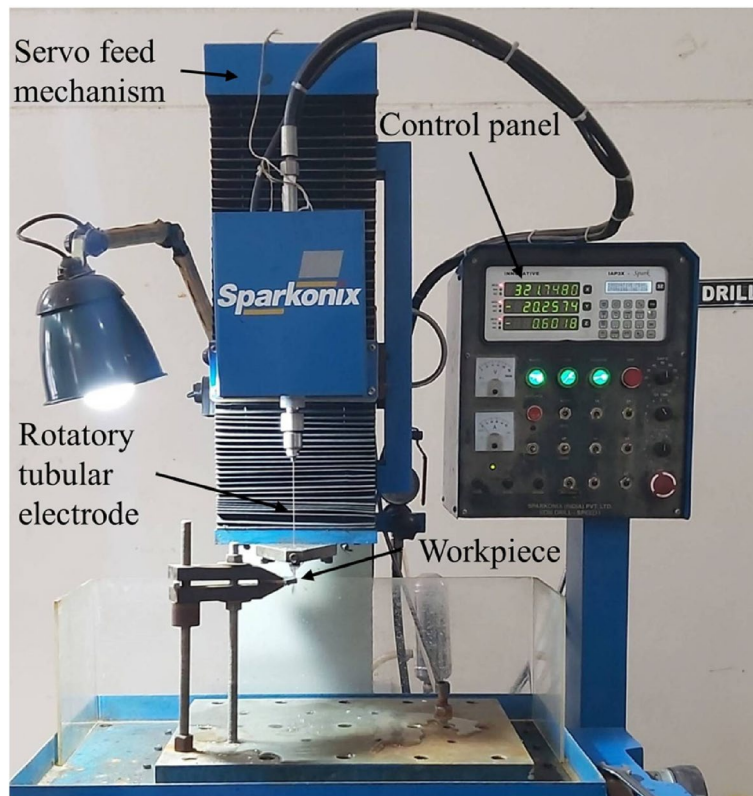
Fig. 2 Photograph of Sparkonix EDM drilling machine
